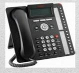
16 line/feature keys with dual LEDs for clear status indication to the user.
