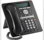
8 line appearance/feature keys with dual LEDs for clear status indication to the user.
